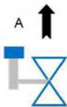
Counterweight mounted on the left (when looking in the flow direction) and dropping in anti-clockwise direction
